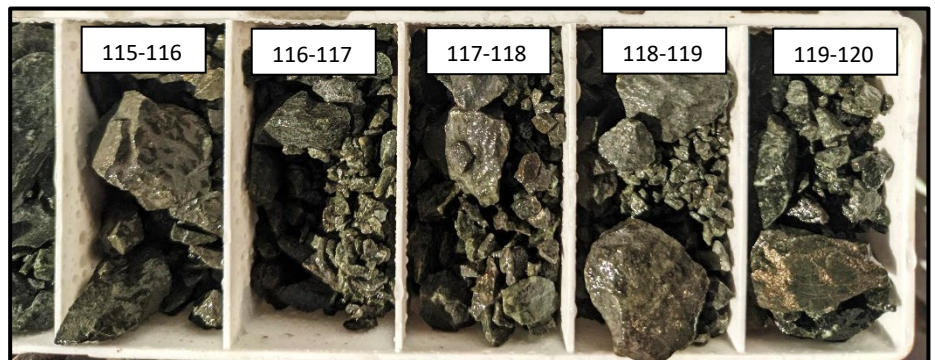
Figure 1 — RC chips with disseminated sulphides (5%) in NRC346
