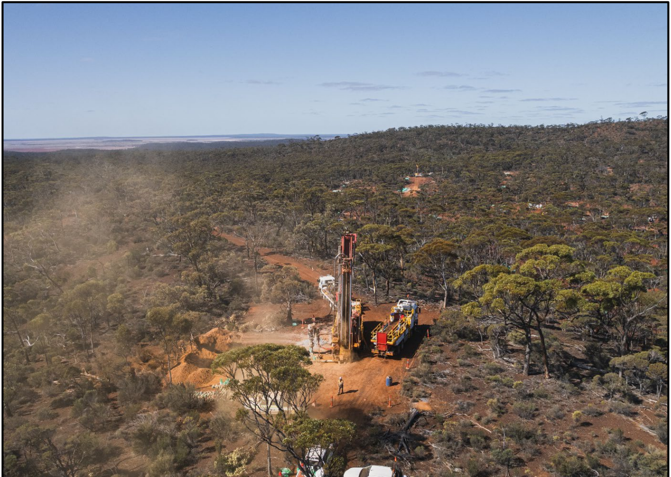
Figure 2 — RC drilling on site at Galileo's 100% owned Norseman project. Diamond drill rig mast is just visible in the background.
