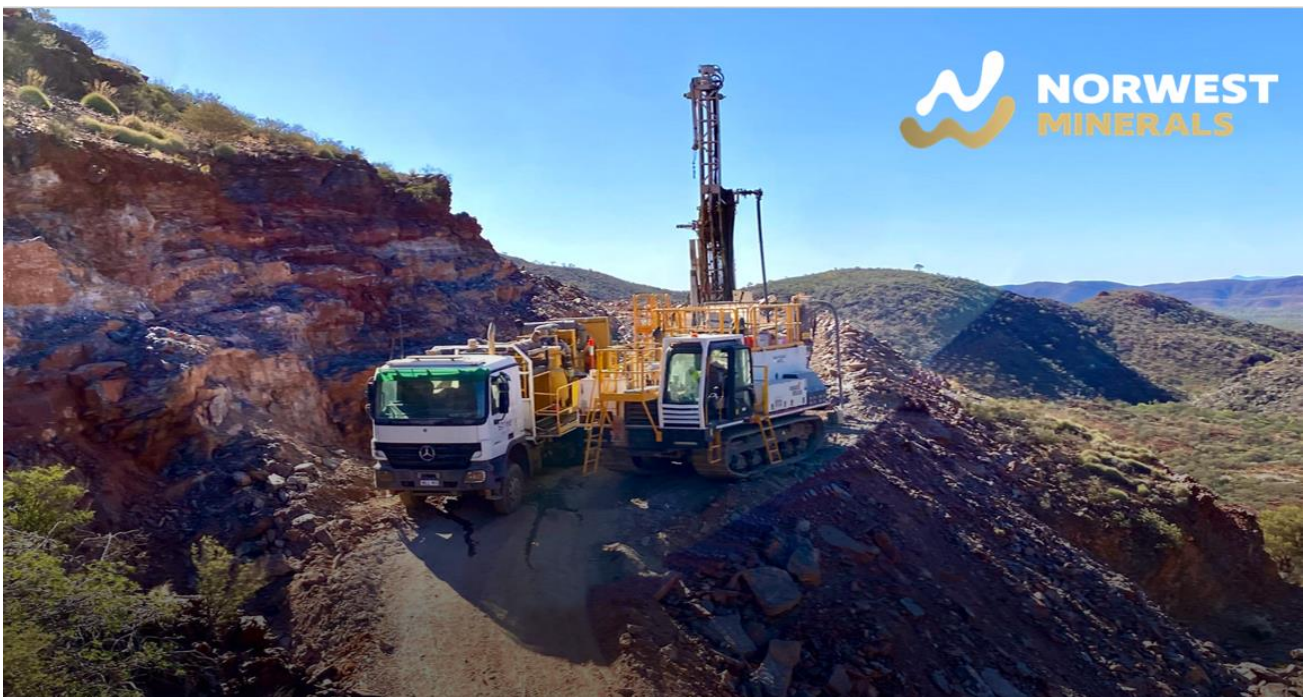
Figure 2 – Strike Drilling's track mounted RC rig at Bali Lo working from drill pad cut into hillside.
