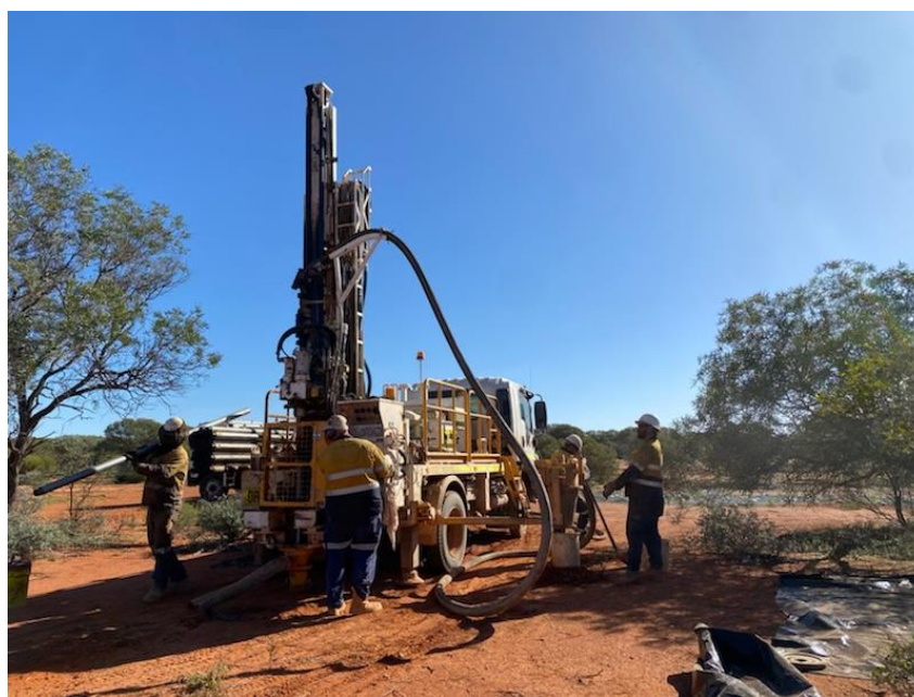
Figure 3. Photo of Seismic Drilling AC drill rig completing the final hole at North Stanmore E 20/871.
