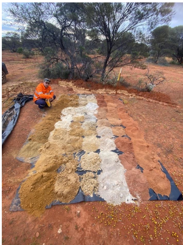
Figure 2. Photo of the samples sorted prior to p-XRF analyses. The colour variation in samples reflects changes in the intensity of weathering and extent of development ionic clays
