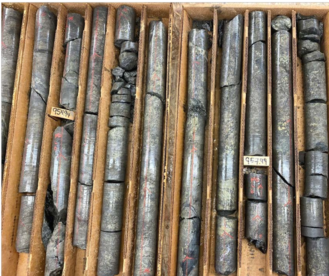
4m of the 13.9m of uninterrupted, very high-grade massive sulphides intersected in drill hole ANT94W3 – the deepest hole drilled yet to test the depth extents of the South Shoot at the Antler Copper Deposit.
