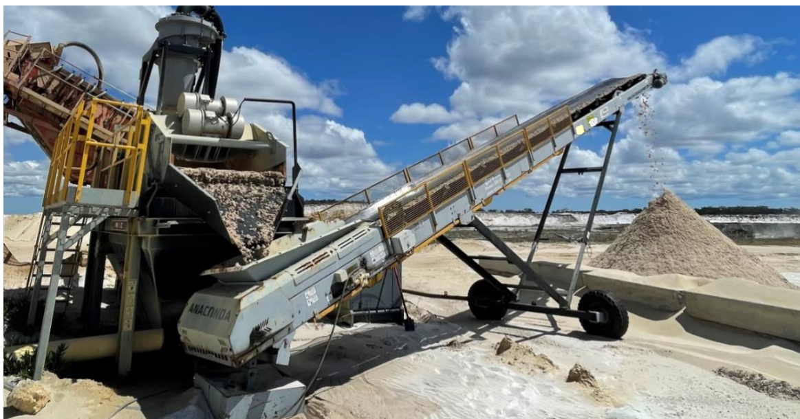
Plate 1. Third party Sand Wash Plant being utilised to process 20 tonne bulk sample from Stockyard Silica Sand Project. Bulk sample is destined for further process beneficiation test work in China at Shandong Hongbote Solar Technology Co., Ltd.
