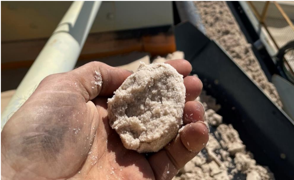
Plate 2. Silica Sand sample after washing, screening, classifying and de-watering.
