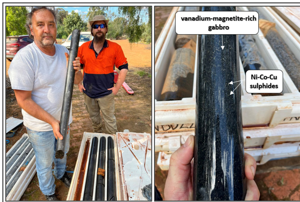
Figure 1 Victory Bore Vanadium Deposit diamond hole VBD2201 drilled for metallurgical testwork (ASX release 18 August 2022), showing vanadium-magnetite bearing core with disseminated sulphides, primarily pyrrhotite (iron sulphide) approximately 2% of the rock mass, with trace (<0.1%) chalcopyrite (copper sulphide) and pentlandite (nickel-cobalt sulphide). Table 1 lists all sulphide visual estimates; the associated cautionary statement also applies to Figure 1.
