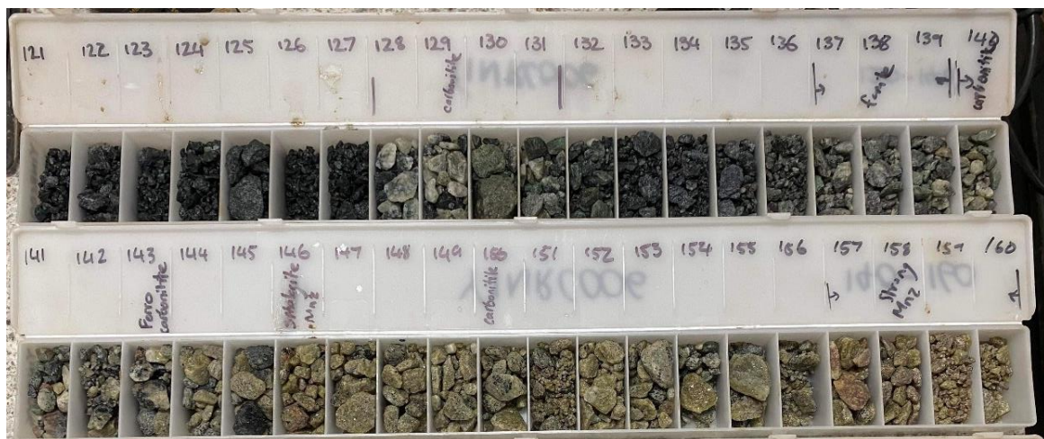
Figure 13: Chip tray from YINRC006 showing dark fenitic alteration grading into two mineralised fresh ironstones (ferrocarnatite) from 127-131m and 139m-160m.
