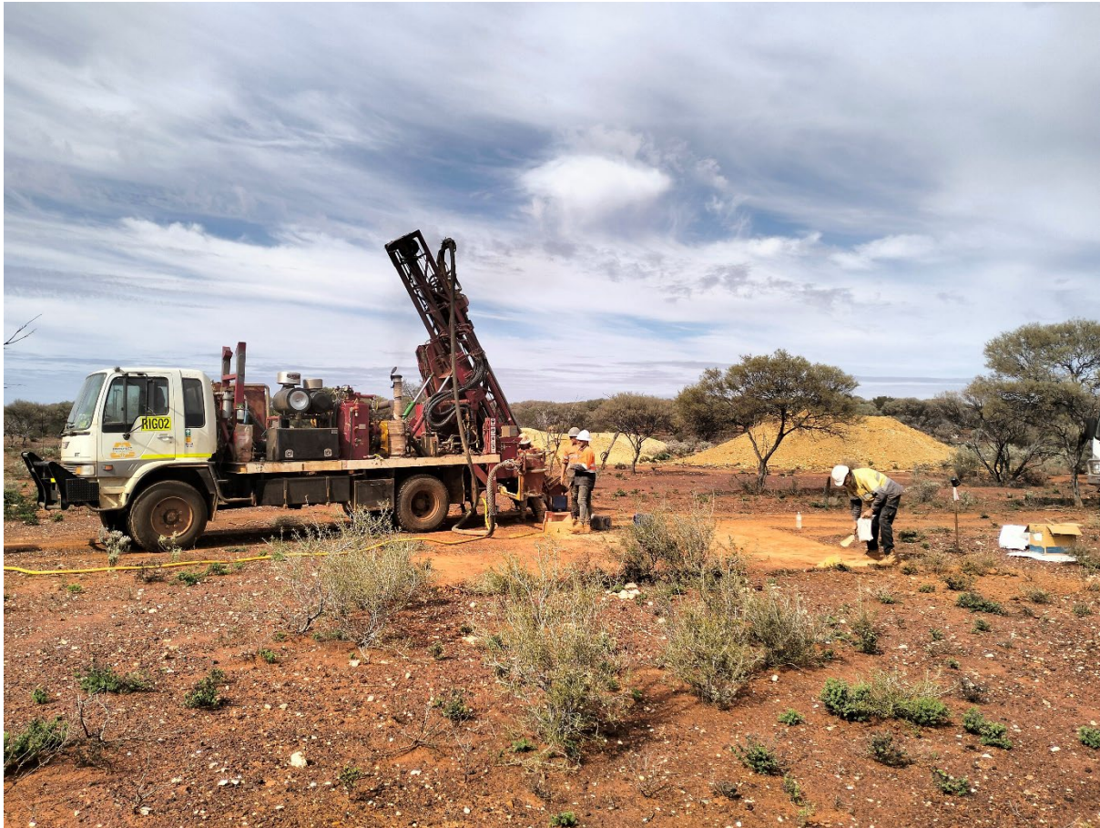
Figure 3: Current aircore drilling at Fred's Well
