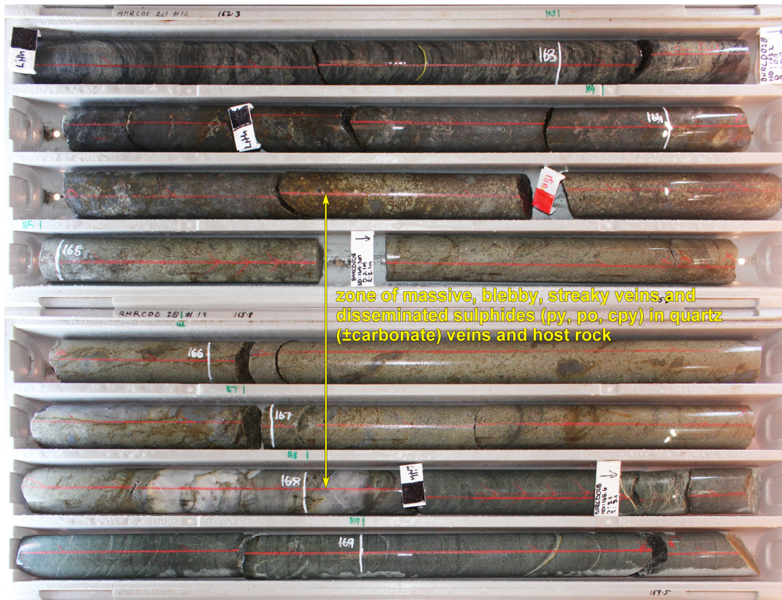
Figure 2: Drill core from 162.3 to 169.5m BHRCD028, showing massive, blebby and disseminated sulphides
