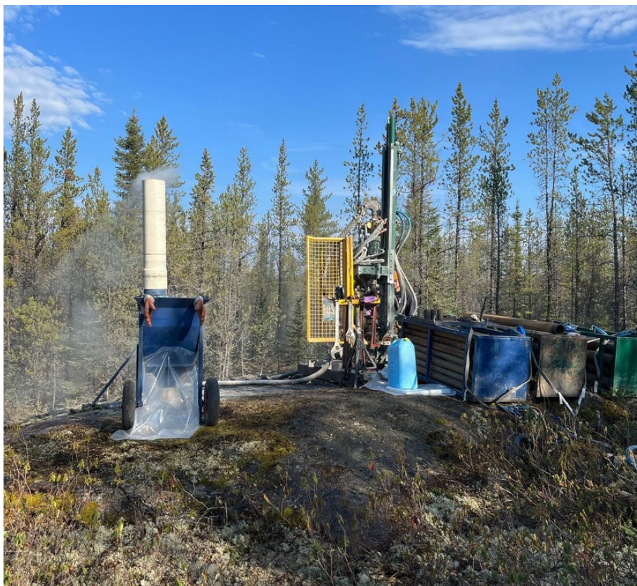
Figure 2: RC drill rig assembled for drilling
