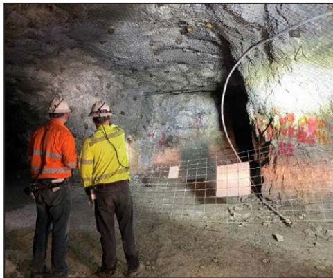
Underground development drive showing good ground conditions
