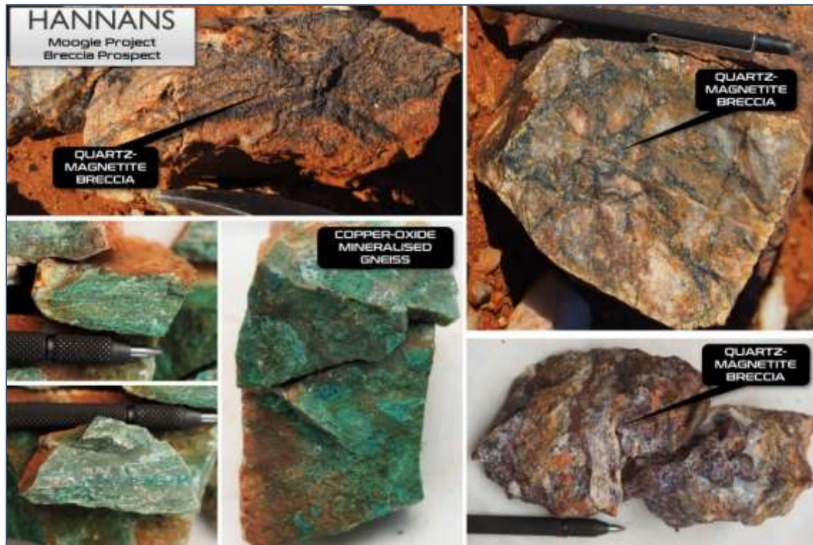
Figure 26: Quartz-magnetite breccia and copper-oxide mineralised gneiss from the Breccia Prospect Source: Outlier Geoscience (2020).
