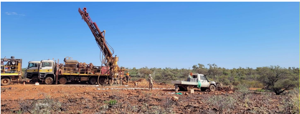
Figure 1: Photo of the RC drill rig fence line drilling at the C3 carbonatite.
