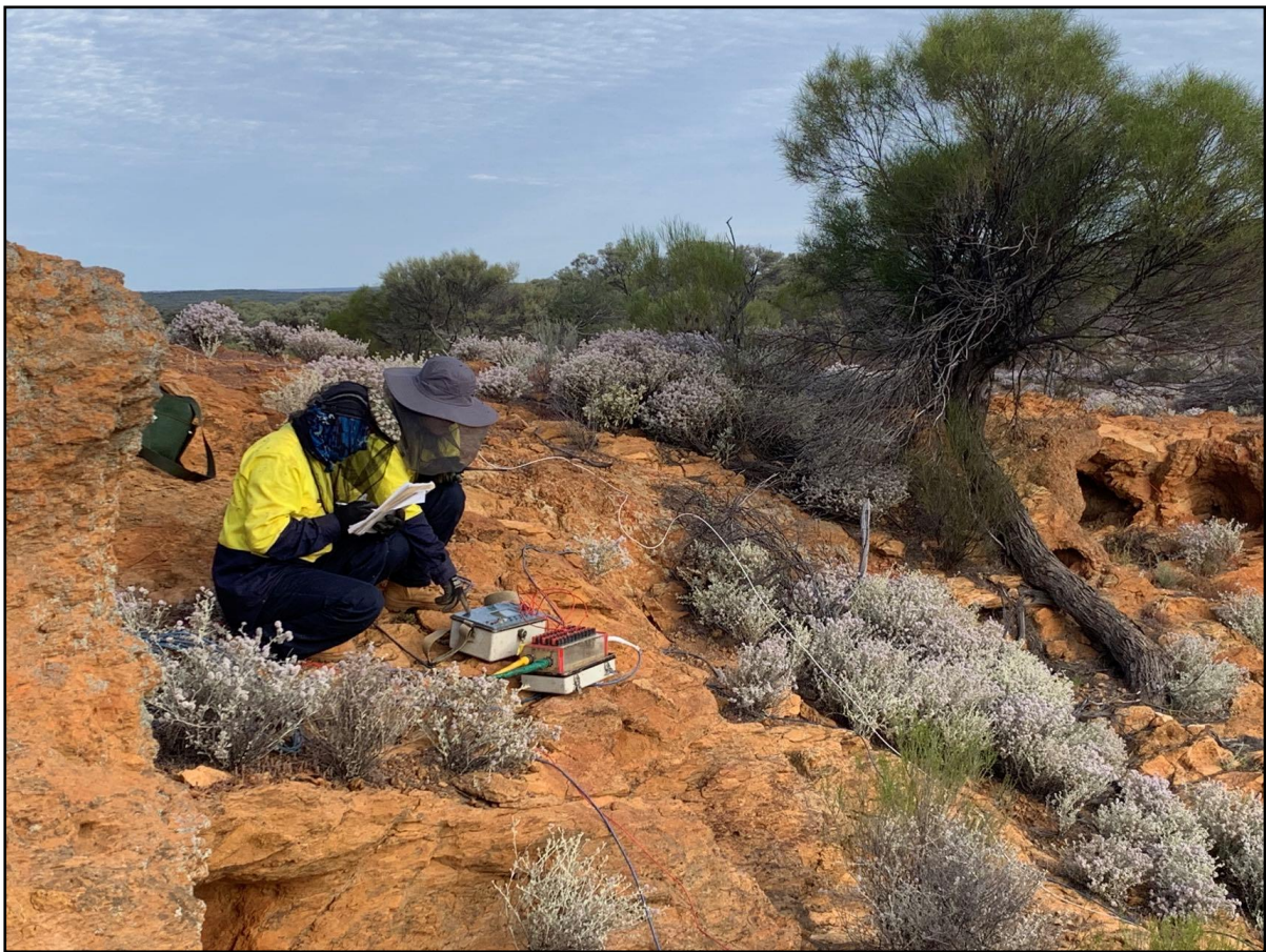
Image of the IP underway at Target 1, currently undertaken by Echo Vista Geophysical Consultants.
