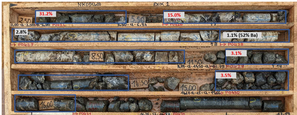
Figure 4 – Mineralisation in NKDD020 – Displaying grades of individual core samples (Zn+Pb%).
