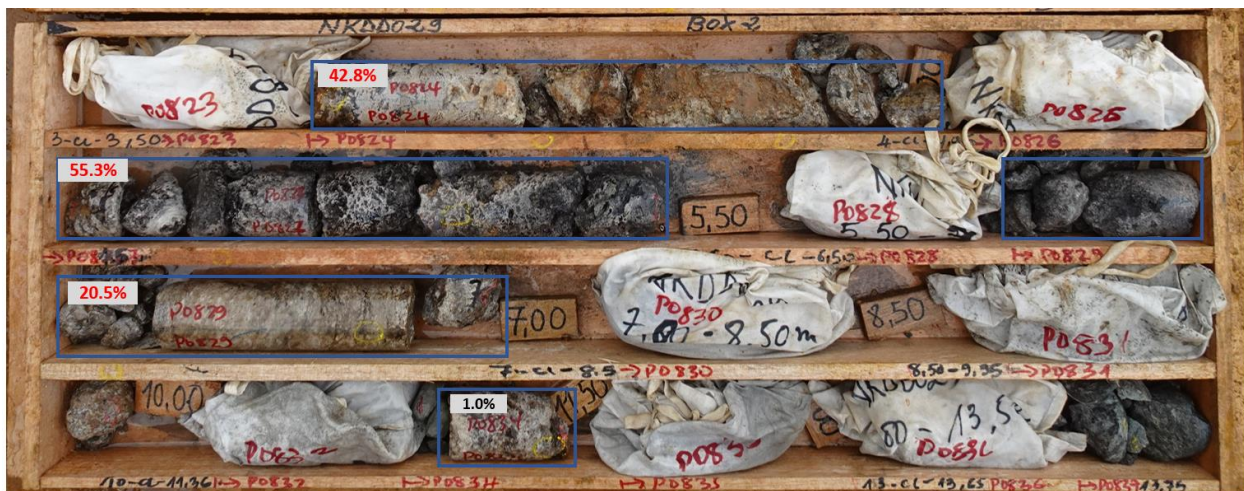
Figure 3 – NKDD029 – Displaying grades of individual core samples (Zn+Pb%).
