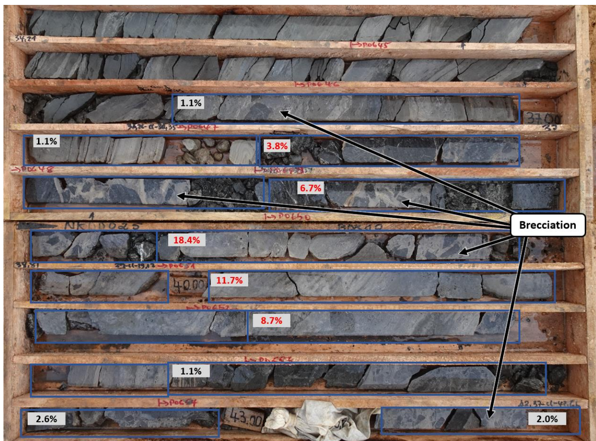
Figure 5 – NKDD025 – Displaying Zn+Pb% grade in core and region of breccia-related mineralisation (36.3m to 45m).
