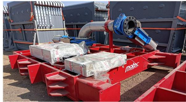
**Pressure filter 2500 – slurry feed distributor**
