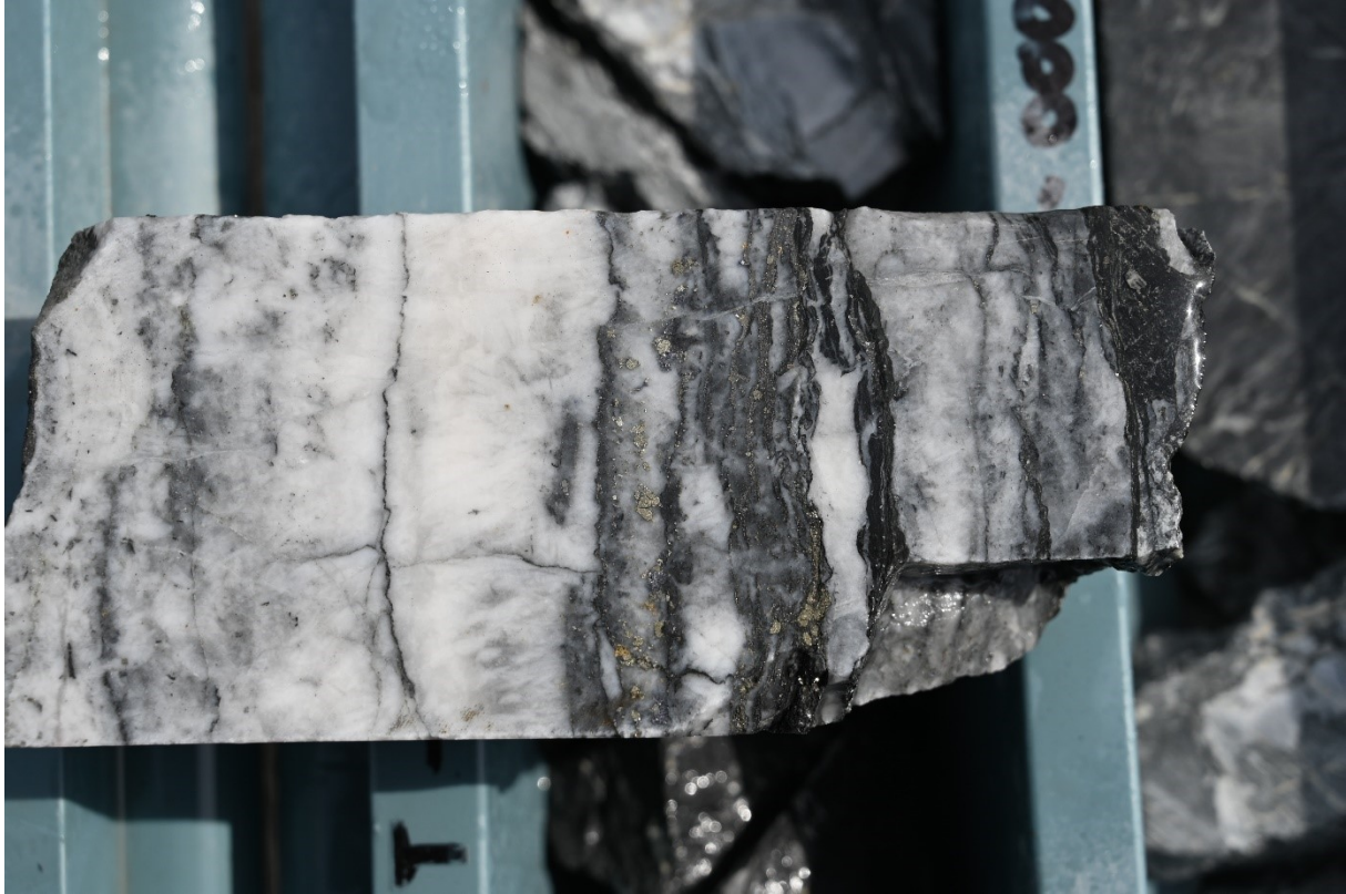
Figure 2 – Example of laminated quartz veining associated with and hosting visible Au. Strong sulphide concentrated along wallrock domains. The quartz laminations vary between milky and sugary to pale grey, translucent and cryptocrystalline. Rare stylolites and tabular, pale grey sugary quartz veins crosscut the laminations at a very high angle
