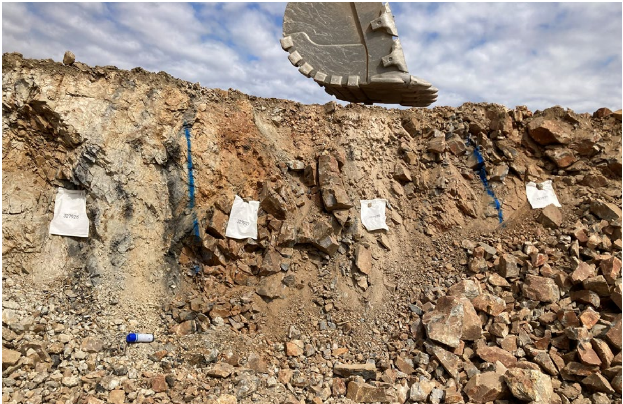
Image 8 - Sampling intervals on a working face.
