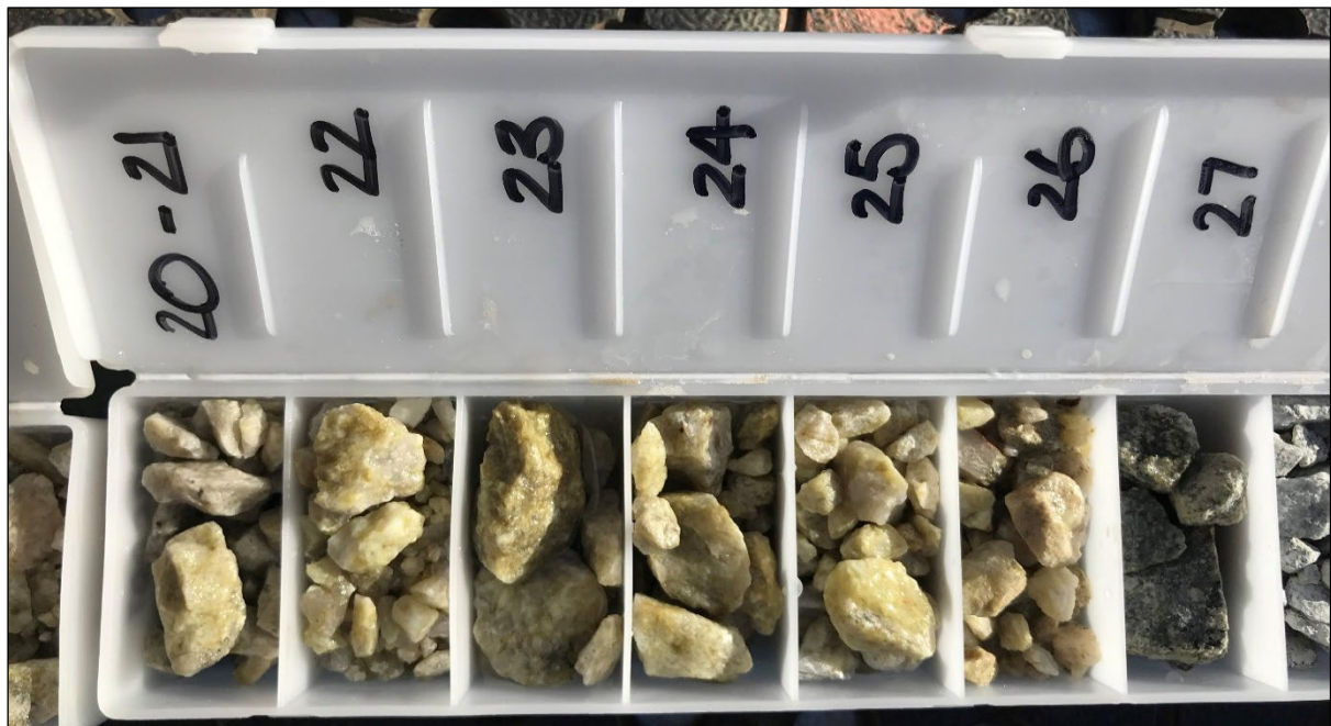
Figure 5 – MBRC007 Drillhole intersecting 6 metres of Pegmatite from 20m to 26m
