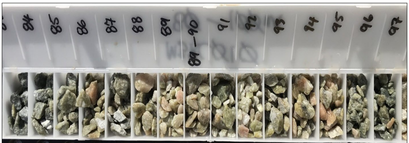
Figure 3 – MBRC010 Drillhole intersecting 9 metres of Pegmatite from 87m to 95m
