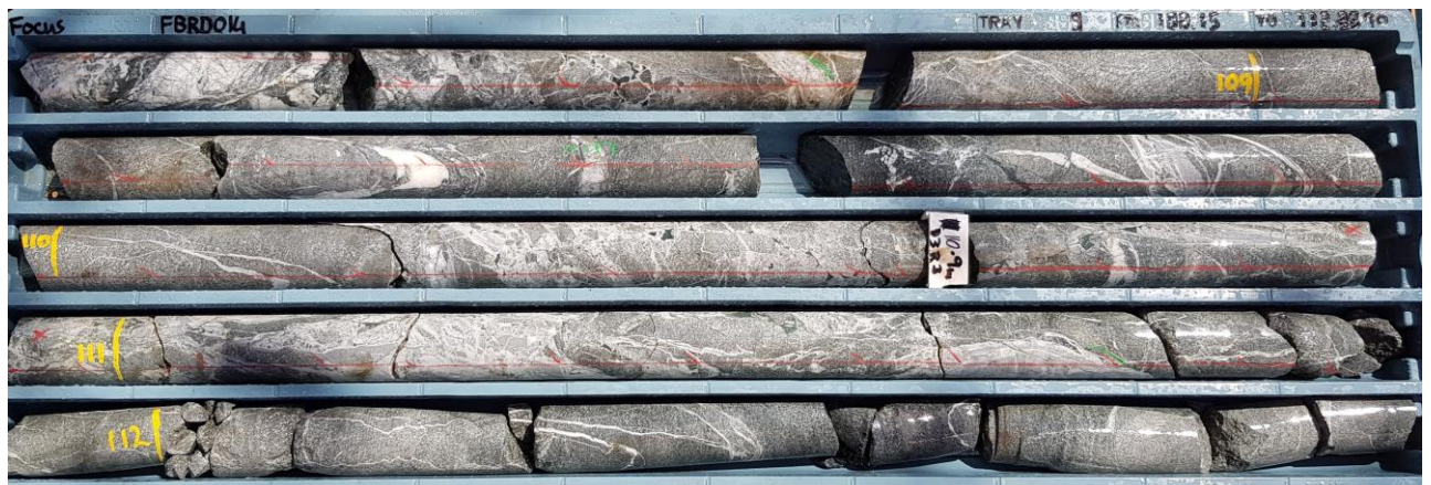
Figure 1: FBRD014 - Intense carbonate veining and brecciation with disseminated chalcopyrite 1 observed between 94 – 110m (tray pictured is 108.15 – 112.7m) – assays pending
