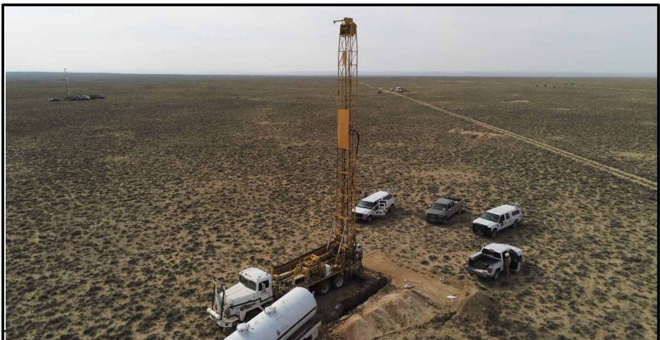
FIGURE 1. MUD ROTARY DRILL RIGS OPERATING, THOR ISR URANIUM PROSPECT, GDB WYOMING.
