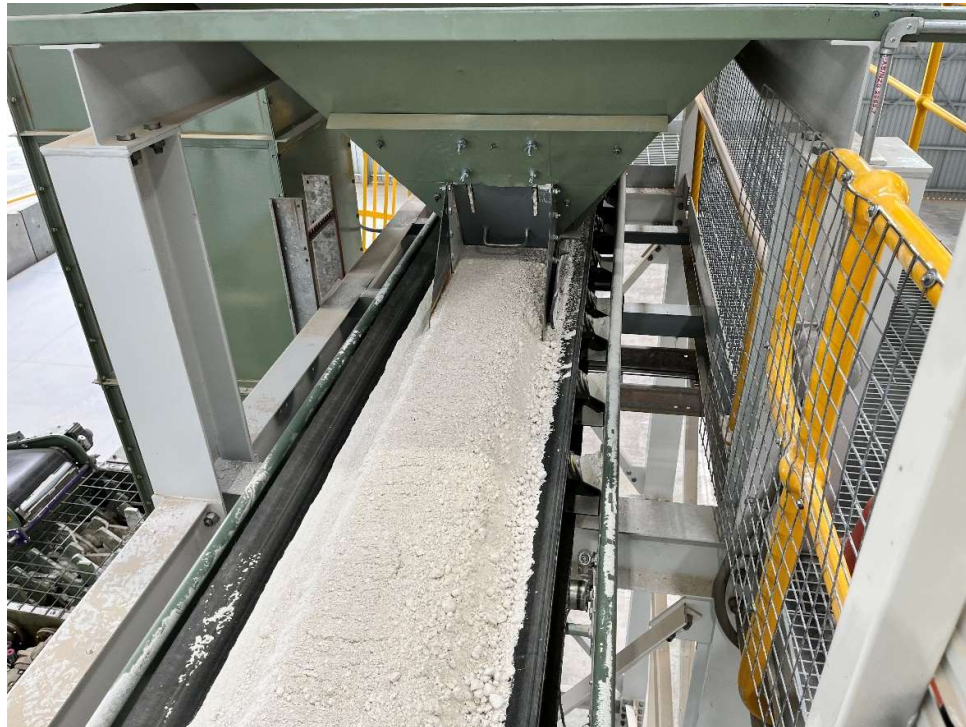
Conditioned ore feed to the rotary kiln September 2022
