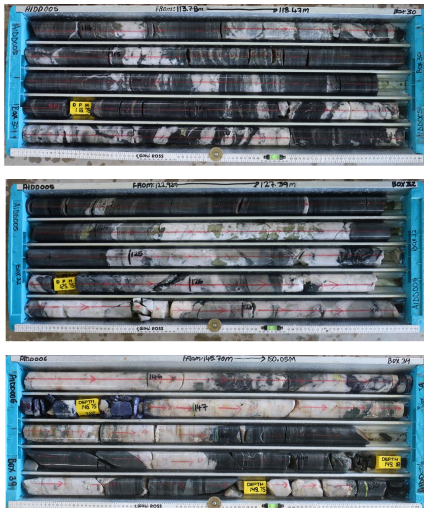
Figure 3: Core photographs characterising the style of mineralisation intersected at A1: (a) A1DD005 - Disseminated chalcopyrite, sphalerite and pyrite associated with quartz-calcite shear-veins; (b) A1DD005 - Chalcopyrite vein-fill; (c) A1DD006 - Semi-massive, vein-in-fill bornite and covellite.
