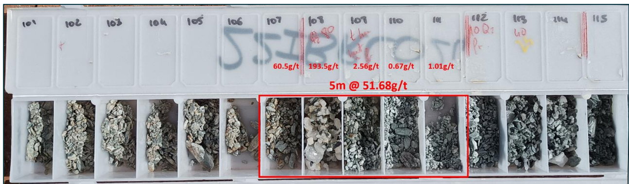
FIGURE 5: RC CHIPS 100 – 115M FROM HOLE 22BRC024. ASSAY PPM VALUES ARE LABELLED IN RED.
