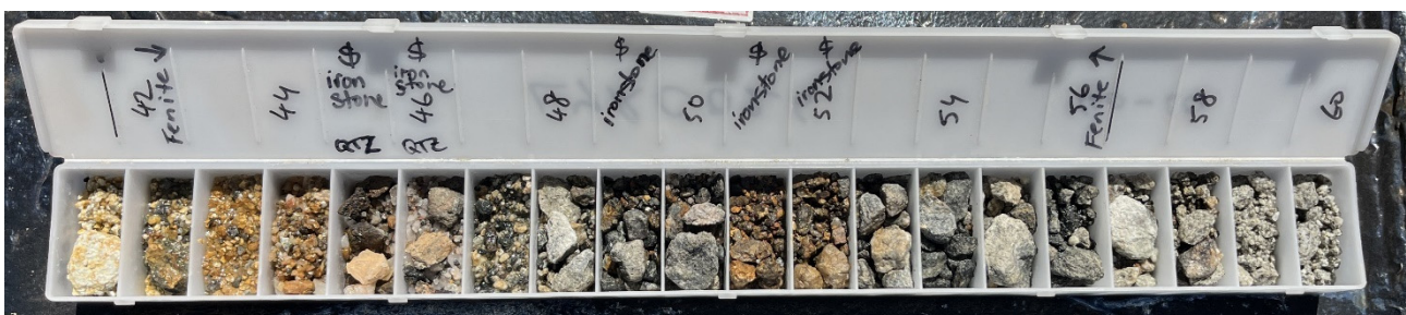
Figure 2. LYRC026 chip tray from the Lyons 12 prospect, intersected two parallel ironstone trends over 2m intervals between 44 – 46m and 50 – 52m, within a broader 15m wide fenitic alteration zone that may potentially be associated with low grade REE mineralisation.
