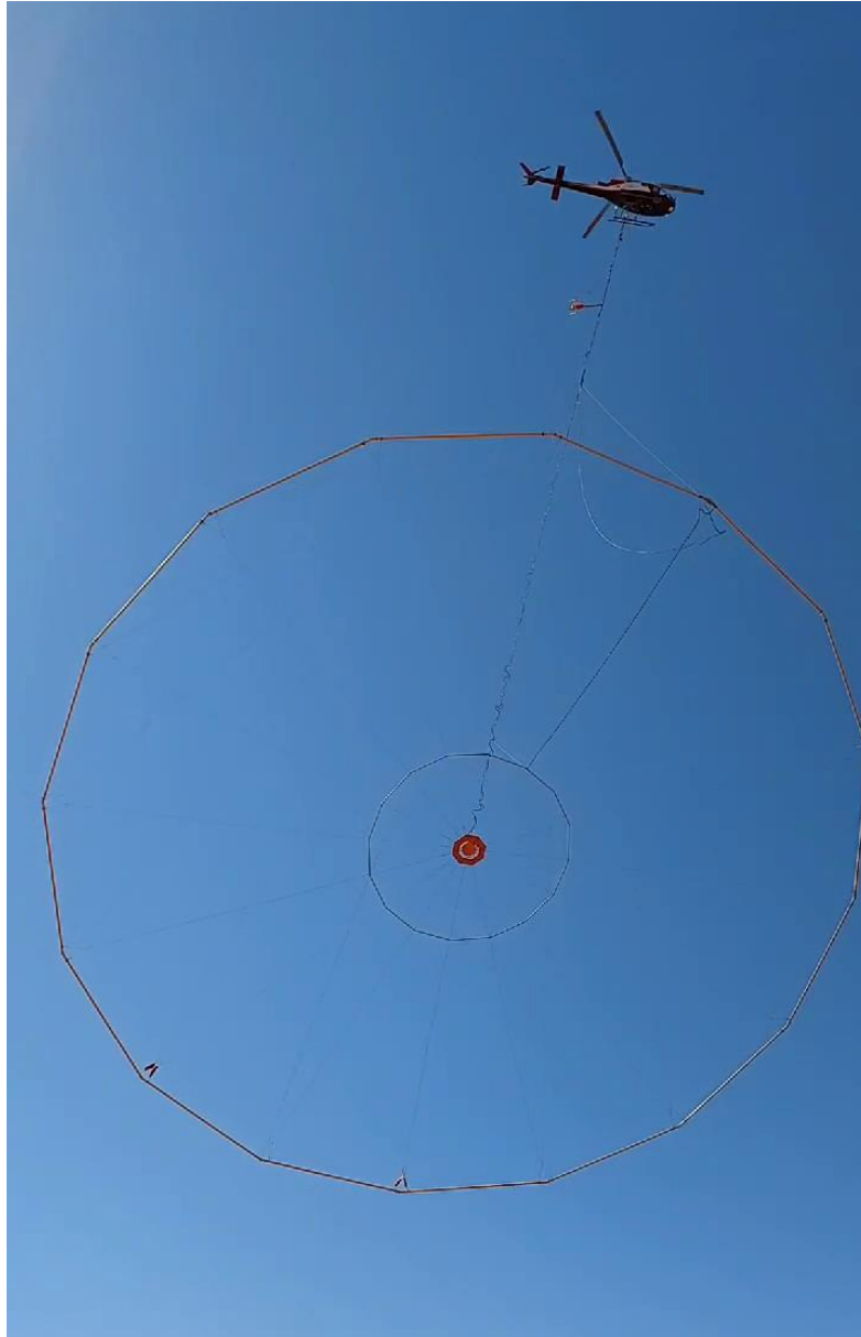
Figure 1 | UTS Geophysics' Helicopter VTEM survey equipment
