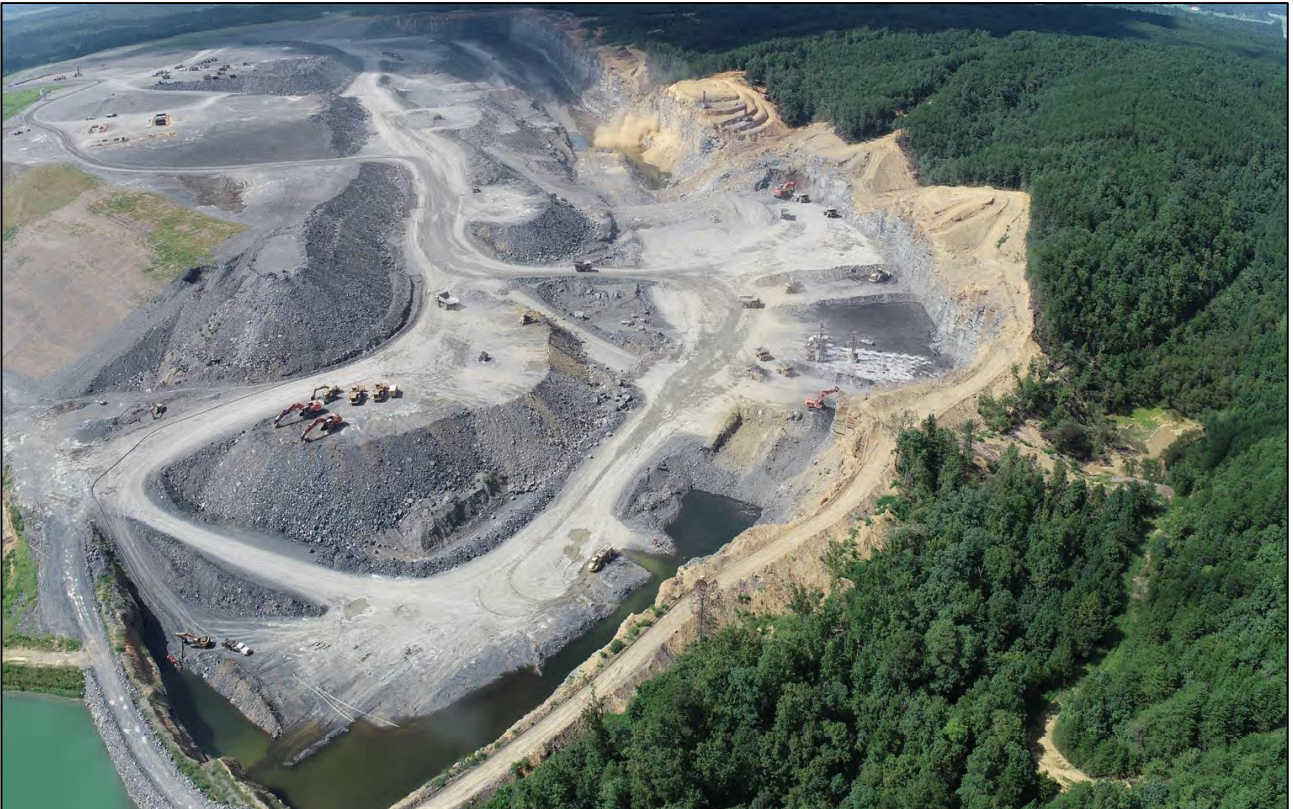
Image: Black Warrior Mine highwall with the flooded pit area to the bottom
