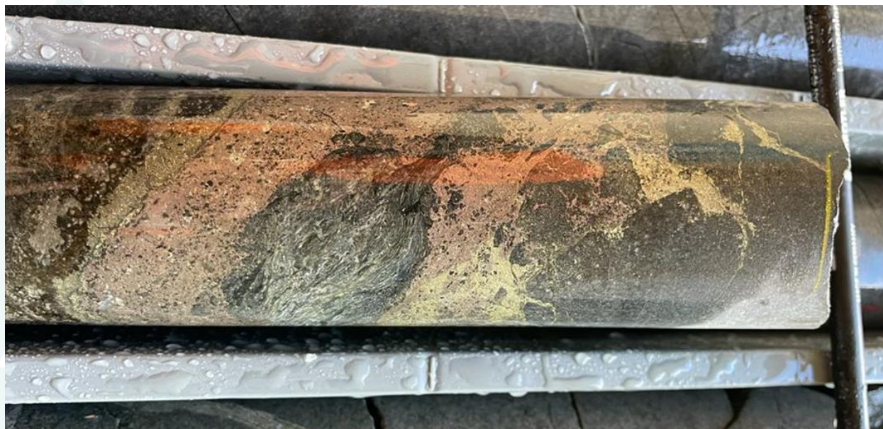
Figure 1: 22B2DD003 (26.8 -27.1 metre interval – NQ core 47.6mm diameter). 0.3m @ 4.14% Ni Eq Strongly mineralised dolerite with fine-grained pyrrhotite, chalcopyrite and coarse minerals of pentlandite. Mineralisation is semi-massive and interstitial.
