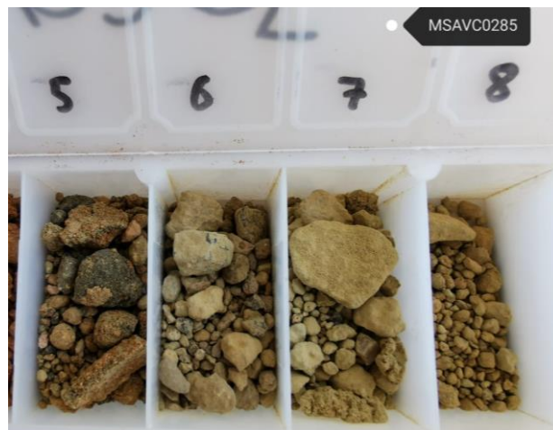
Photo 2: MSAVC0285 with 4m @ 474ppm TREYO + 65ppm Sc 2 O 3 from 4m; inc 1m @ 636ppm TREYO + 52ppm Sc 2 O 3 from 5m
