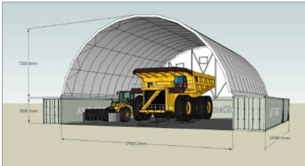
Figure 25: Example of Double-container height Haulpak workshop.
