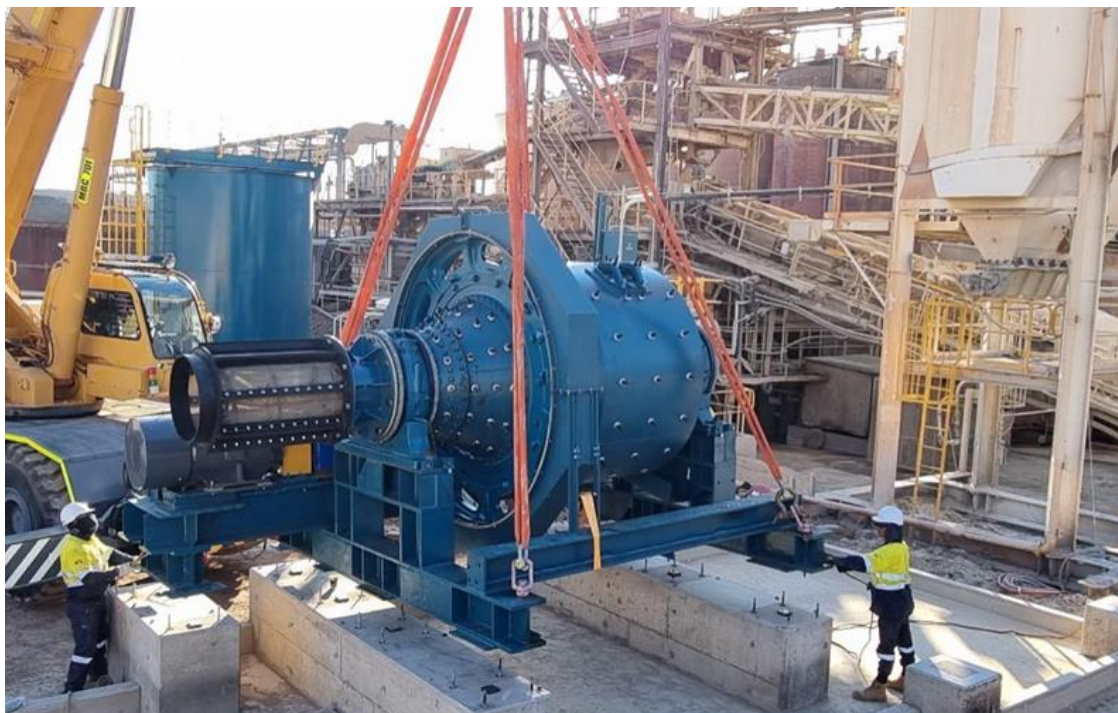
Figure 4: Refurbished Lime Slaking Mill for Wiltails
