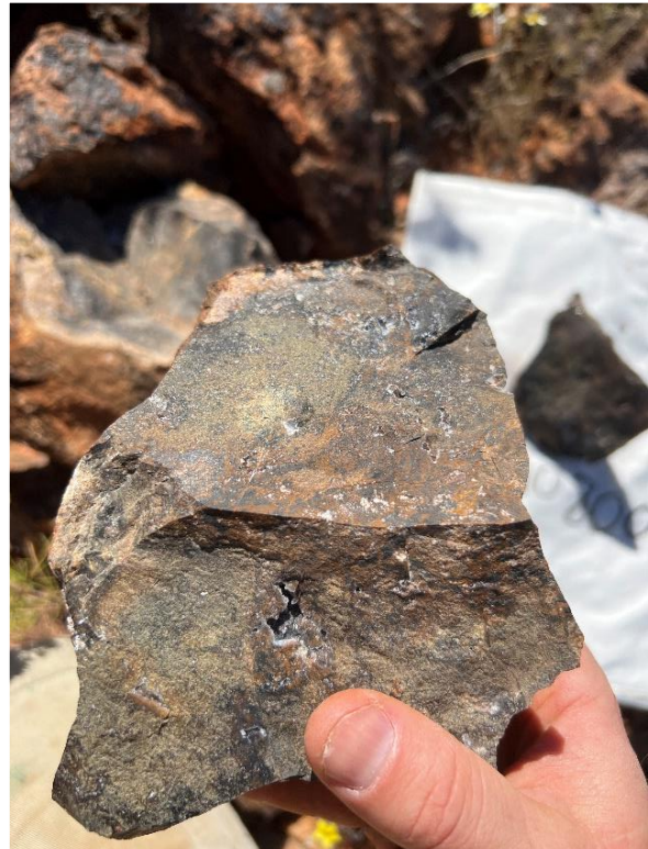
Figure 9: High grade monazite-rich samples MWGS1114 (left) and monazite rich sample MWGS0800 (right) which assayed 15.79% TREO with 2.41% \text{Nd}_2\text{O}_3 + \text{Pr}_6\text{O}_{11} and 13.30% TREO with 1.99% \text{Nd}_2\text{O}_3 + \text{Pr}_6\text{O}_{11} .
