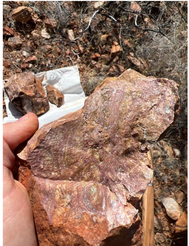
Figure 7: Massive monazite sample MWGS1108 (left) and MWGS0848 (right) which assayed 28.07% TREO with 4.63% \text{Nd}_2\text{O}_3 + \text{Pr}_6\text{O}_{11} and 23.81% TREO with 3.97% \text{Nd}_2\text{O}_3 + \text{Pr}_6\text{O}_{11} .
