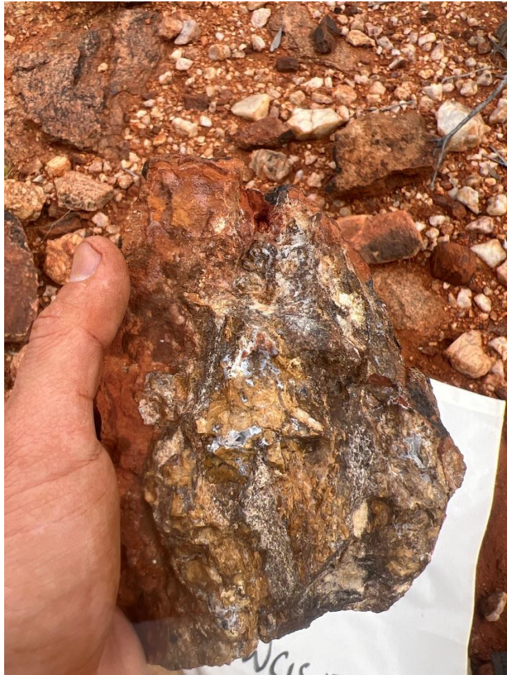
Figure 11: Monazite-rich rock chip sample MWGS1224 which assayed 17.64% TREO with 3.82% \text{Nd}_2\text{O}_3 + \text{Pr}_6\text{O}_{11} .
