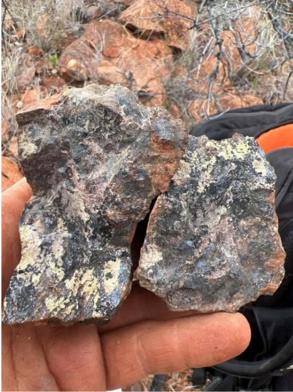
Figure 8: Monazite (pale red) rich carbonatite samples MWGS0769 (left) and MWGS0770 (right) which assayed 21.55% TREO with 3.74% \text{Nd}_2\text{O}_3 + \text{Pr}_6\text{O}_{11} and 15.19% TREO with 2.56% \text{Nd}_2\text{O}_3 + \text{Pr}_6\text{O}_{11} .
