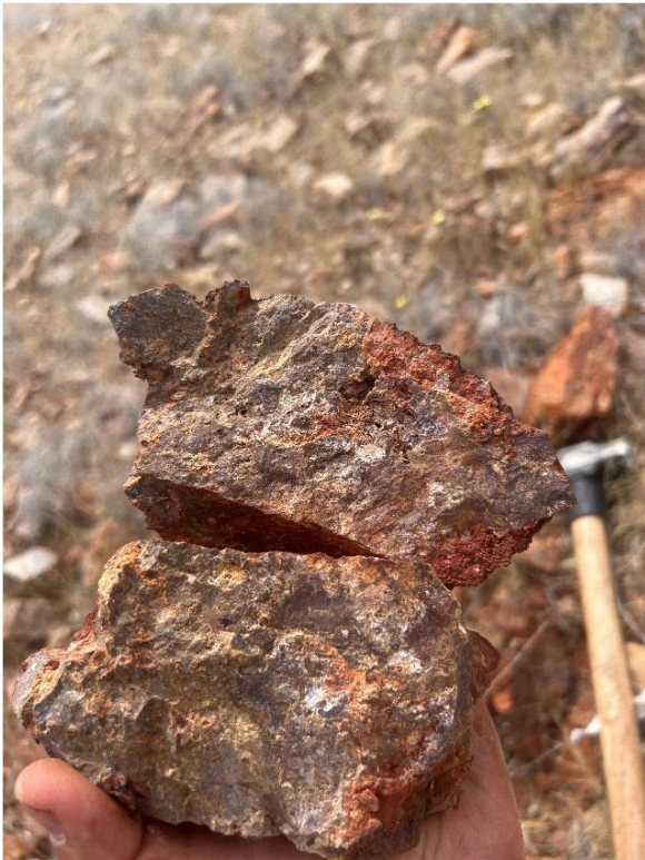
Figure 9: High grade monazite-rich samples MWGS1114 (left) and monazite rich sample MWGS0800 (right) which assayed 15.79% TREO with 2.41% \text{Nd}_2\text{O}_3 + \text{Pr}_6\text{O}_{11} and 13.30% TREO with 1.99% \text{Nd}_2\text{O}_3 + \text{Pr}_6\text{O}_{11} .
