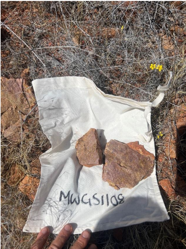
Figure 7: Massive monazite sample MWGS1108 (left) and MWGS0848 (right) which assayed 28.07% TREO with 4.63% \text{Nd}_2\text{O}_3 + \text{Pr}_6\text{O}_{11} and 23.81% TREO with 3.97% \text{Nd}_2\text{O}_3 + \text{Pr}_6\text{O}_{11} .
