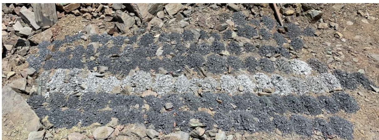
Figure 2. HMHSRC001 chip piles. The sulphidic interval is associated with quartz and can be seen as the lighter coloured chip piles.
