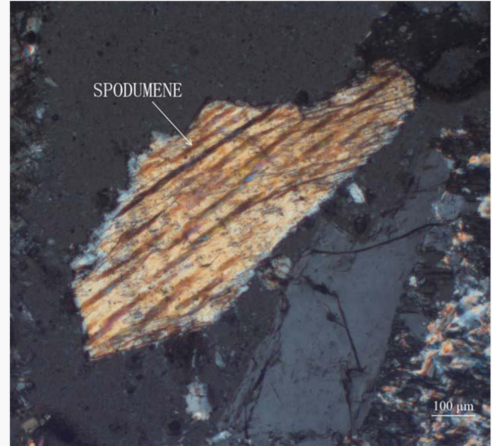
Electron microscope image of a lithium bearing spodumene monocrystal from the Marble Bar metallurgical test work.
