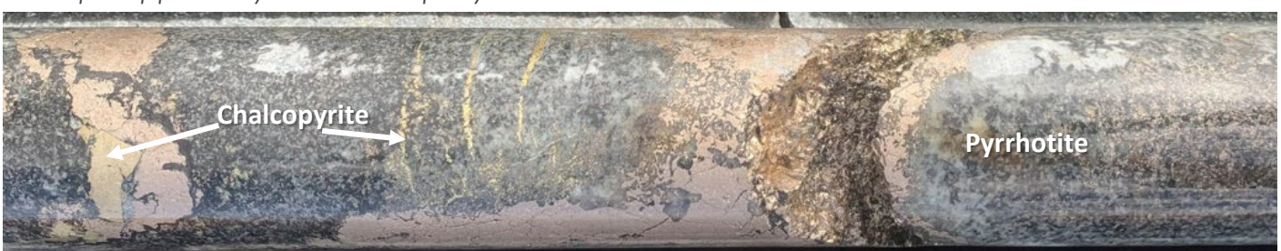
Figure 1. Massive sulphides in TMDD0001, chalcopyrite, pyrrhotite and pyrite observed, 841m depth.
