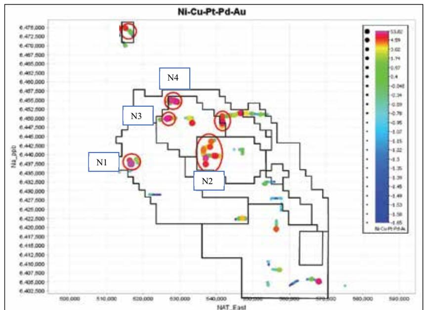
**Figure 1.2:** Additive Z scores for Ni-Cu-Pd-Pt-Au across the main Arkun project area. Note the large areas of anomalism in the central part of the project area. Four priority areas for follow up work are highlighted. Other areas of elevated response are also evident including the Beau target to the north.
