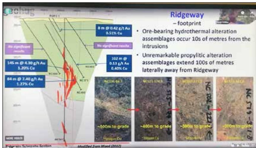
**Figure 7.3:** Summary of the geology and copper values around the Ridgeway deposit located near Orange in NSW. Note the very low levels of copper present in so called "unremarkable" altered rocks even as close as 200 metres to 300 metres away from the high grade core (RHS of Figure). Distinctive alteration halos only occur within 10's of metres thick around high grade zones. The cross section shows a deposit would be easily missed unless the drill spacing was about 200 metres between holes.
