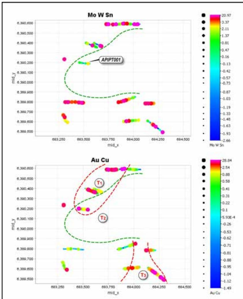
**Figure 7.4:** Maps showing the down hole traces of drill holes showing metal assemblages for copper-gold (Cu-Au core) and molybdenum-tungsten-tin (Mo-W-Sn upper phyllic zone) at Apsley. Three target areas for follow up work have been identified (T1, T2 and T3).
