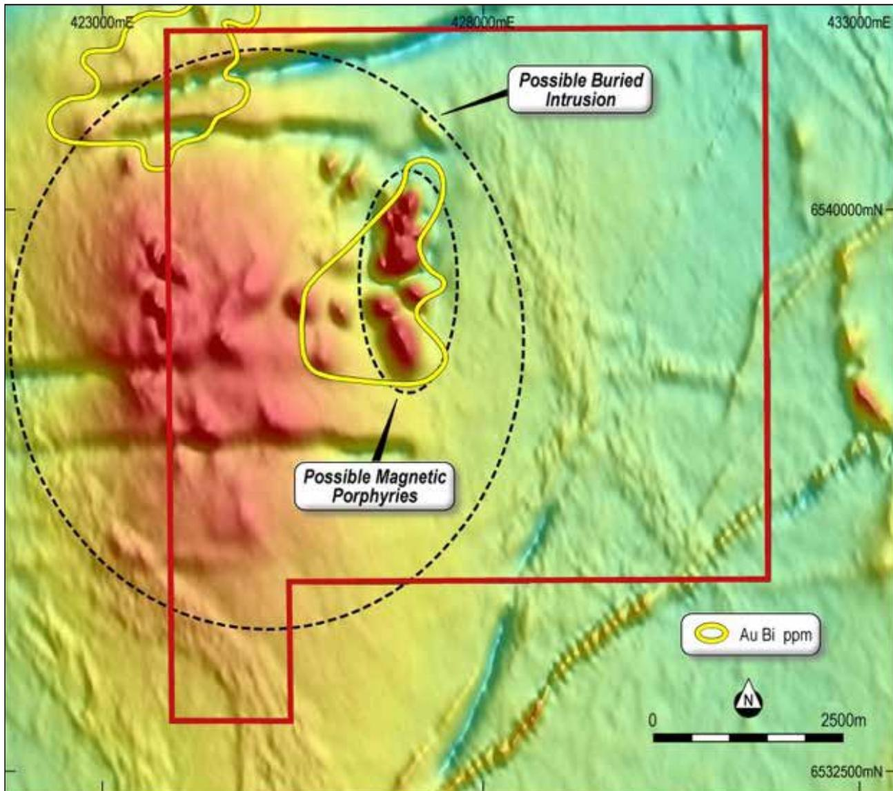
**Figure 5.2:** Image of regional magnetic data over the Doonia project with warmer colours indicating more magnetic units. A large oval deep-seated anomaly is centred directly under the project area above which a cluster of near surface anomalies is present and interpreted as possible magnetic intrusions. These smaller anomalies are coincident with a gold-bismuth soil geochemistry anomaly (ASX Release 17<sup>th</sup> November 2020).
