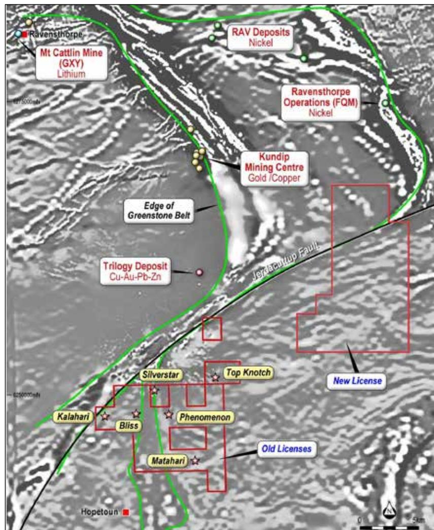
**Figure 4.1:** Image of airborne magnetic data over the Ravensthorpe-Hopetoun area showing the interpreted extension of the Ravensthorpe greenstone belt south of the Jerdacuttup Fault together with the licences in the Hopetoun Joint Venture. The new licence is EL74/730.
