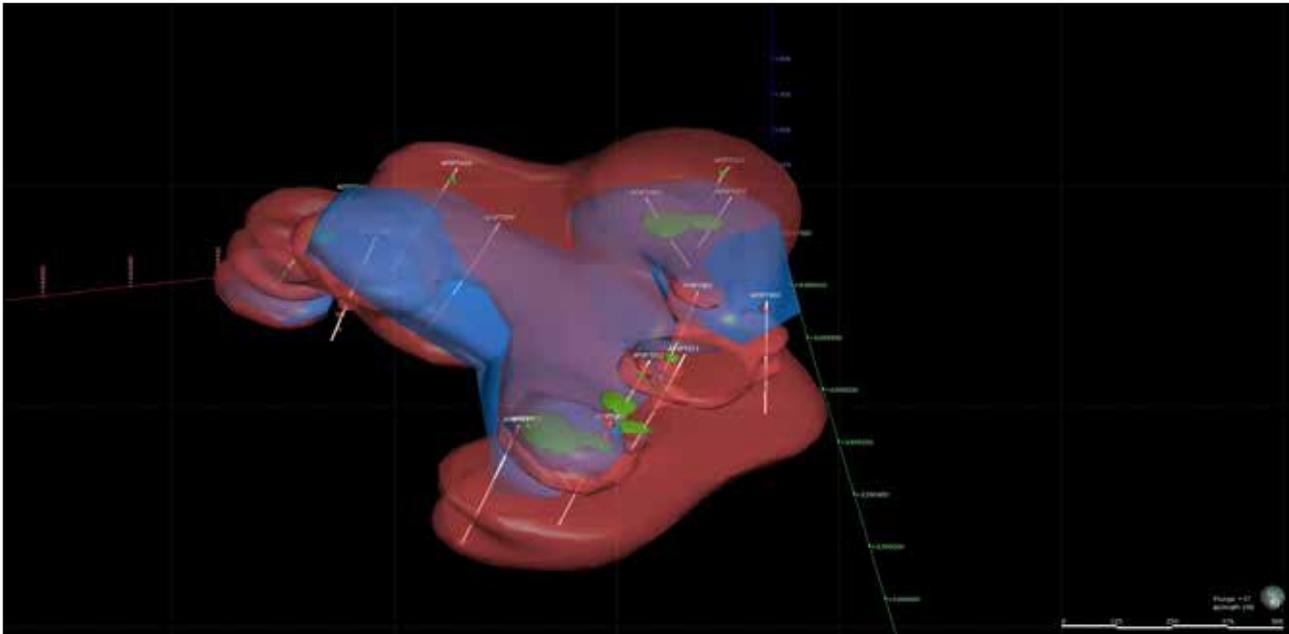
**Figure 7.2:** View looking South of the copper halo (red bubbles >100 ppm copper, green bubbles >200 ppm copper) with an associated molybdenum halo (>2 ppm molybdenum). Thick intercepts of low to modest grade copper occur over an area of at least about one square kilometre.
