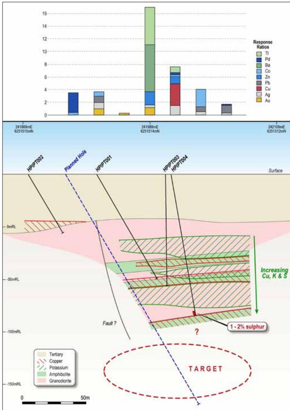
**Figure 4.2:** Cross section from the Top Knotch Prospect showing the soil geochemistry responses and highlighting the sub-horizontal zones of alteration and copper which are increasing in intensity down hole. The location of the one off completed diamond drill holes is also shown.
