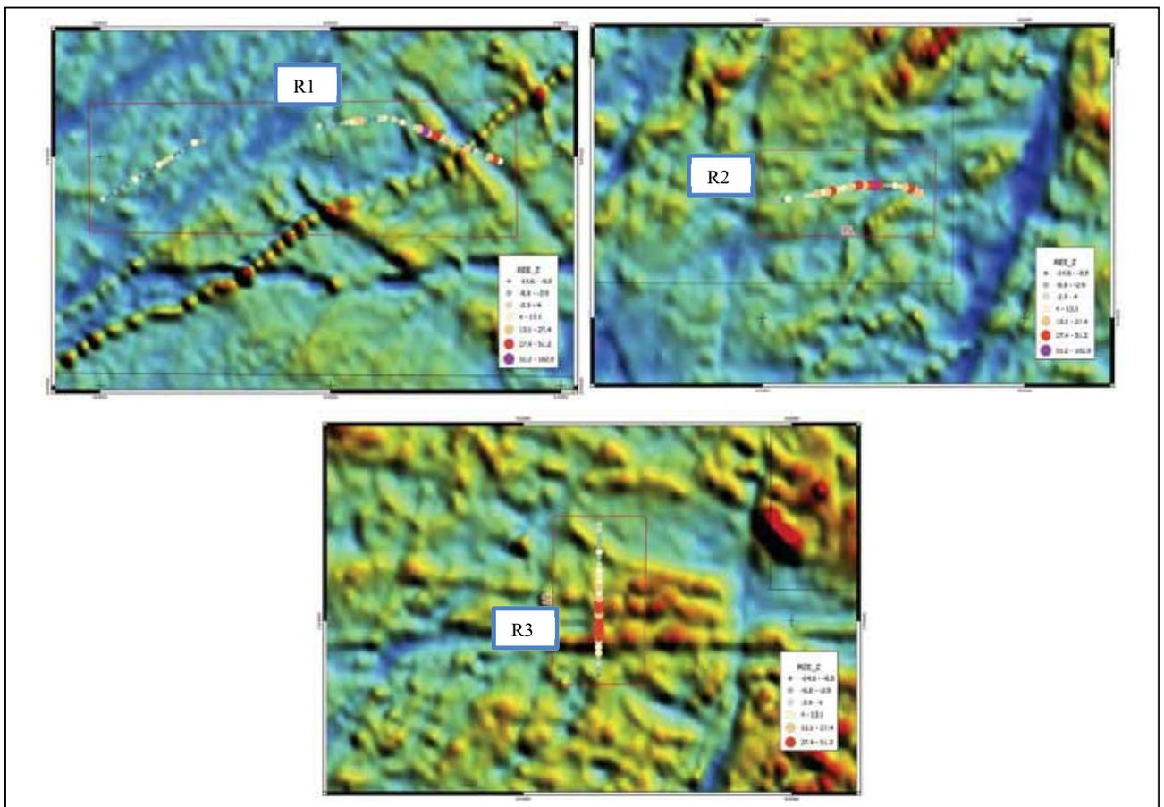
**Figure 1.8:** Priority Targets for REE shown on images of regional magnetic data. Strongly elevated soil geochemistry responses extend over distances of many hundreds of metres and are mainly associated with the magnetic units with larger granite bodies.
