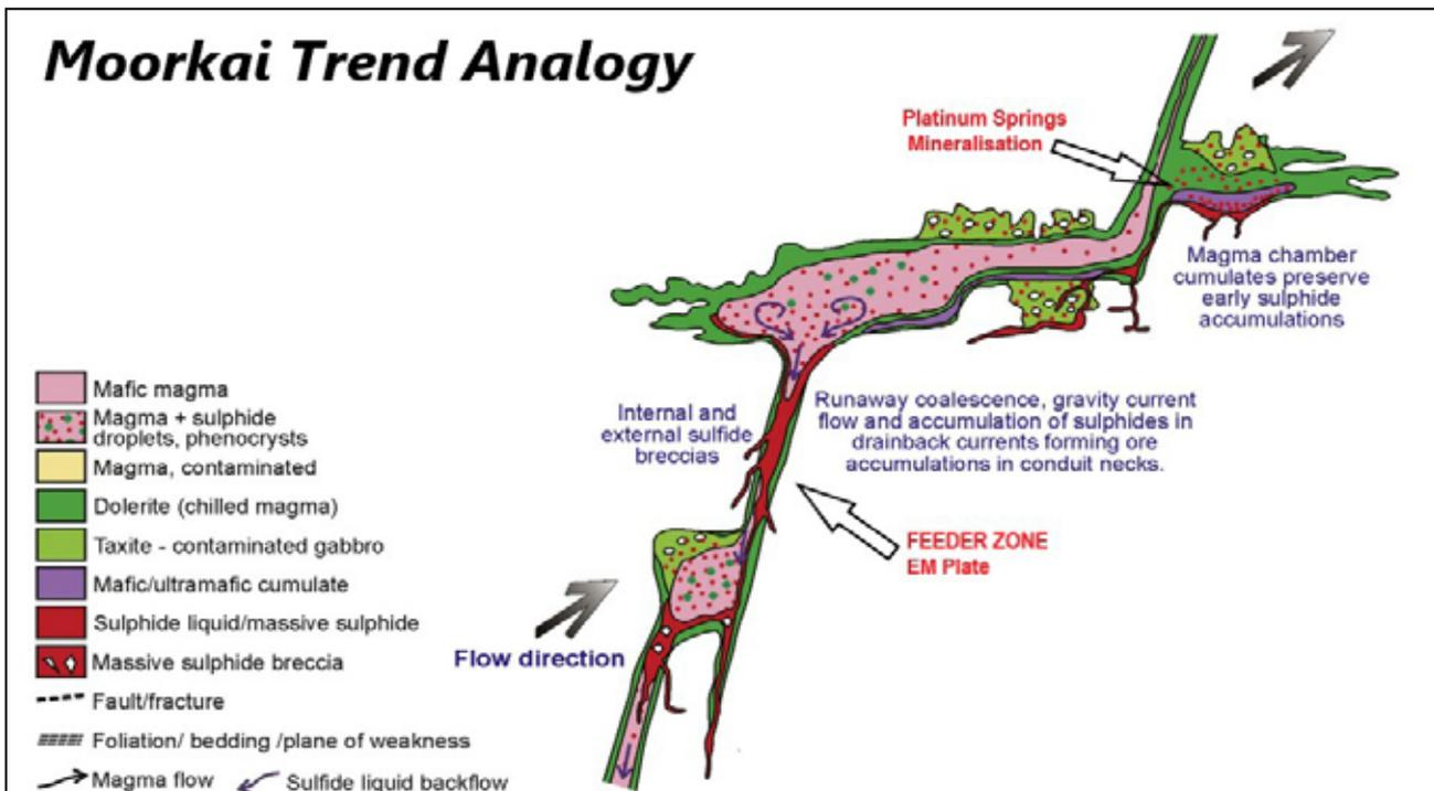
**Figure 6.5:** Model for the formation of nickel-copper-PGM deposits within evolving magma conduits including chonoliths. Note the massive sulphide within the feeder zones/conduit necks (from Barnes, S.J. et al. Ore Geology Reviews Volume 76, July 2016, Pages 296-316)
