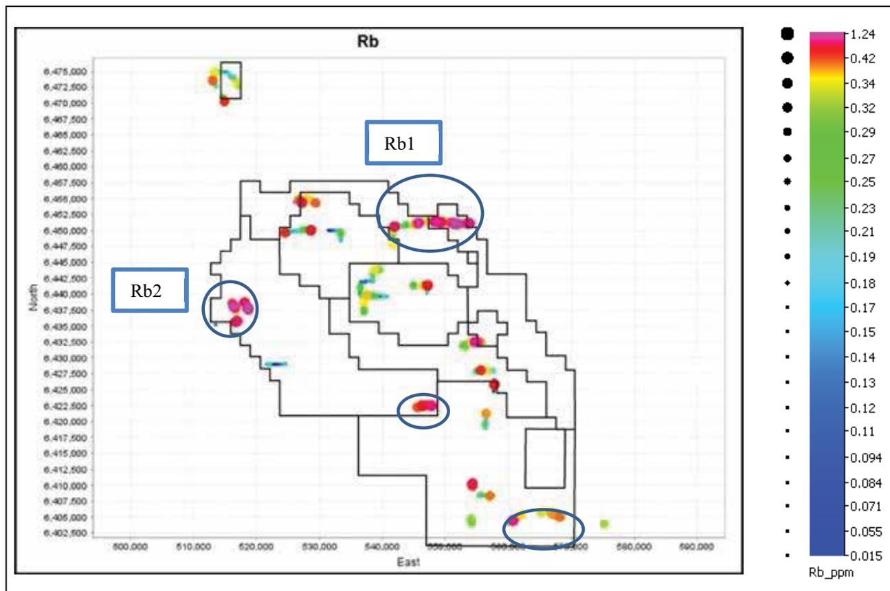
**Figure 1.7:** Ionic leach results for rubidium. Four priority areas for follow up work are highlighted. Other areas of elevated response are also evident. Note that the low absolute levels of rubidium are a function of the very dilute nature of the chemical digest used in the Ionic Leach assay method.
