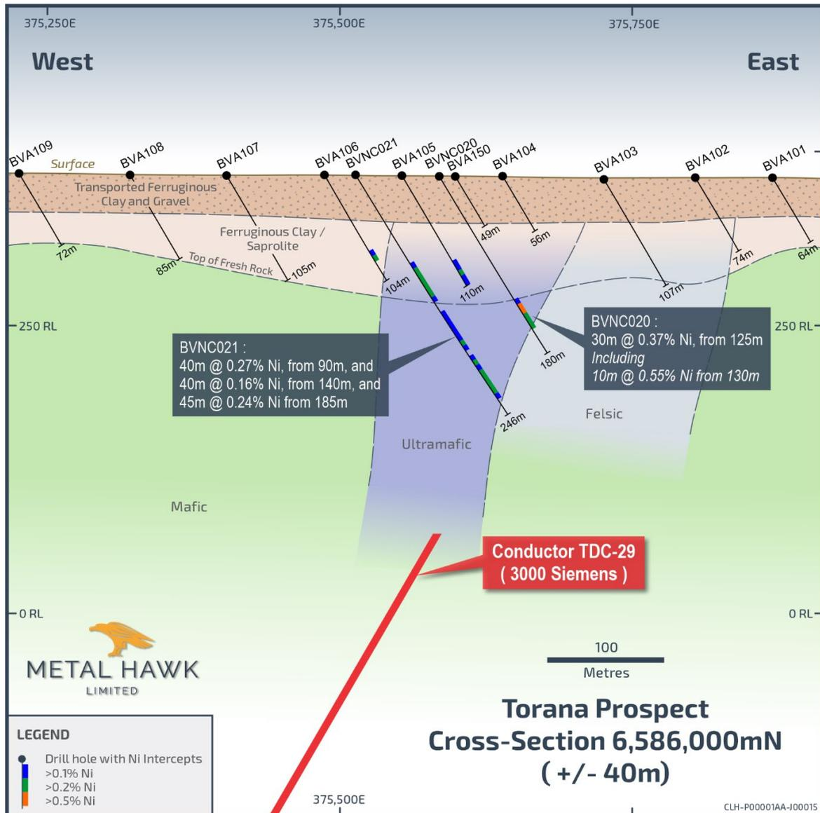
**Figure 4.** Torana Prospect – cross-section showing DHEM target **TDC-29**
