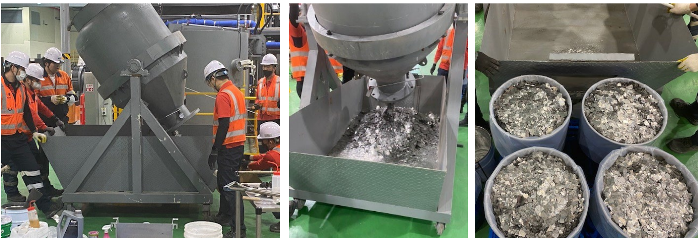
Neodymium iron boron (NdFeB) strip caster and product at the Korean Metals Plant
