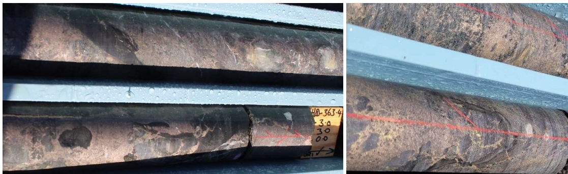
Photo 1: Massive/matrix breccia sulphides, 363m. Photo 2: Massive/matrix breccia sulphides, 351m.
