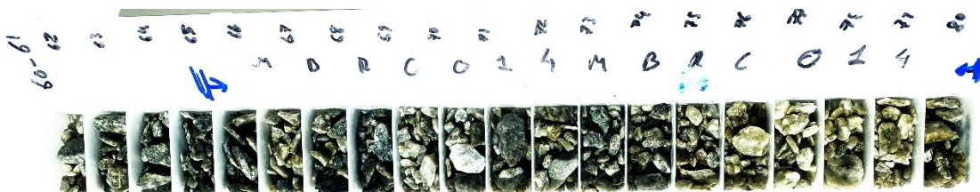
Figure 5 – MBRC014 Drillhole intersecting 14 metres of altered Pegmatite from 65m to 79m
