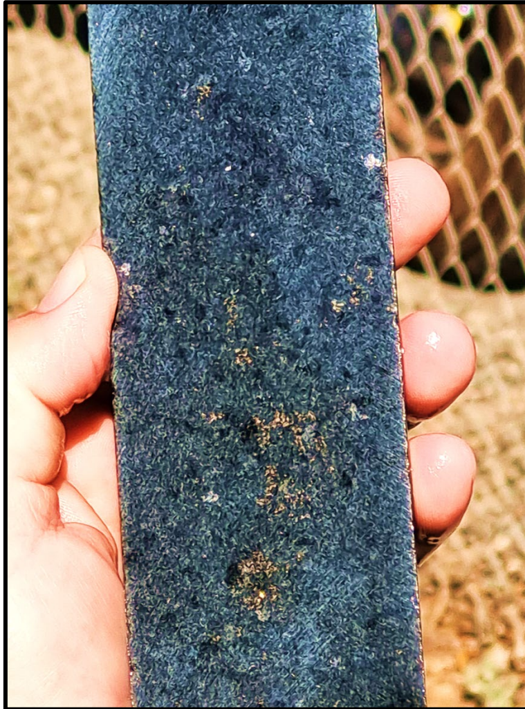
Figure 1 – Example of disseminated sulphide mineralisation in cut drill core from Callisto. Estimated sulphides are typically 3% to 5% over individual metres. NRCD279 at approximately 250m down hole, drill core diameter is 51mm.
