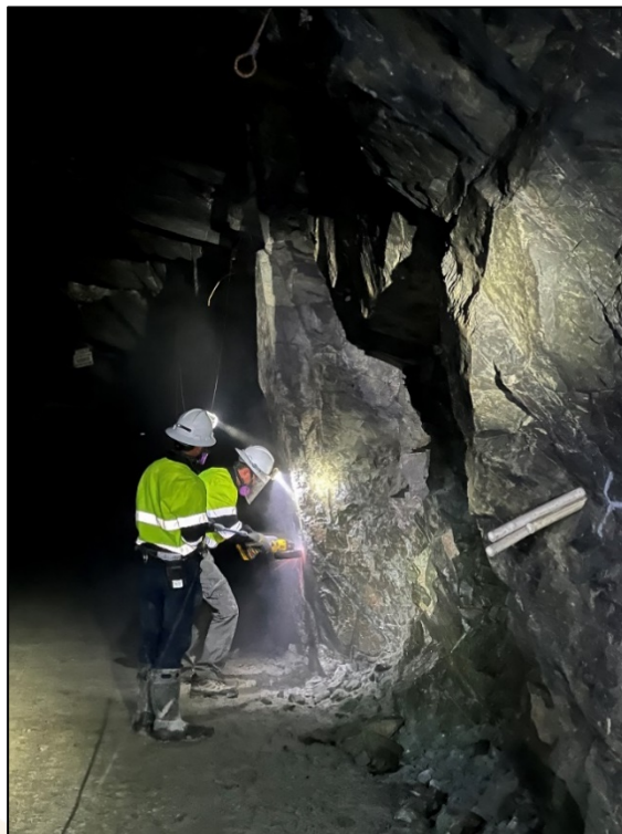
Photo 7 - Channel Sampling of Mineralised zones from underground
