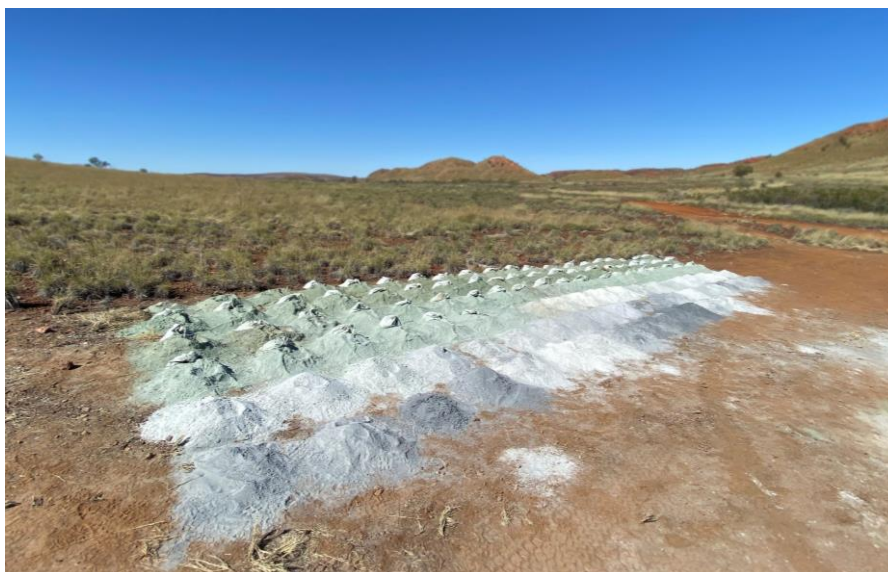
Photo 2: 22RRC010 drill spoils showing the strong 'white' sericite altered zone from approximately 73m with
