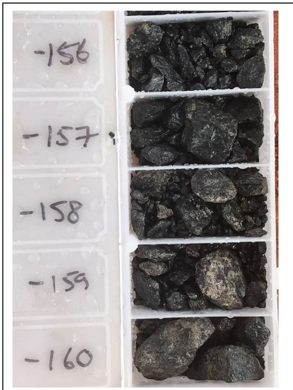
Image 1 / RC drill chips: 22SKRC001 146m to 165m, Gabbro with stringer pyrrhotite/pyrite/chalcopyrite. 19m at 5,000 ppm Cu, 1,297 ppm Ni, 100 ppm Co, 0.28 ppm Pd, 0.11 ppm Pt
