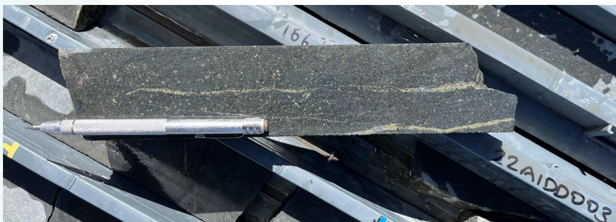
Figure 2: 22A1DD003 (156 - 165 metre interval – NQ core 47.6mm diameter). Strongly mineralised dolerite with fine-grained disseminated pyrrhotite-chalcopyrite mineralisation (note the chalcopyrite veining), within a 20.8 metre zone of sulphide mineralisation. 1
