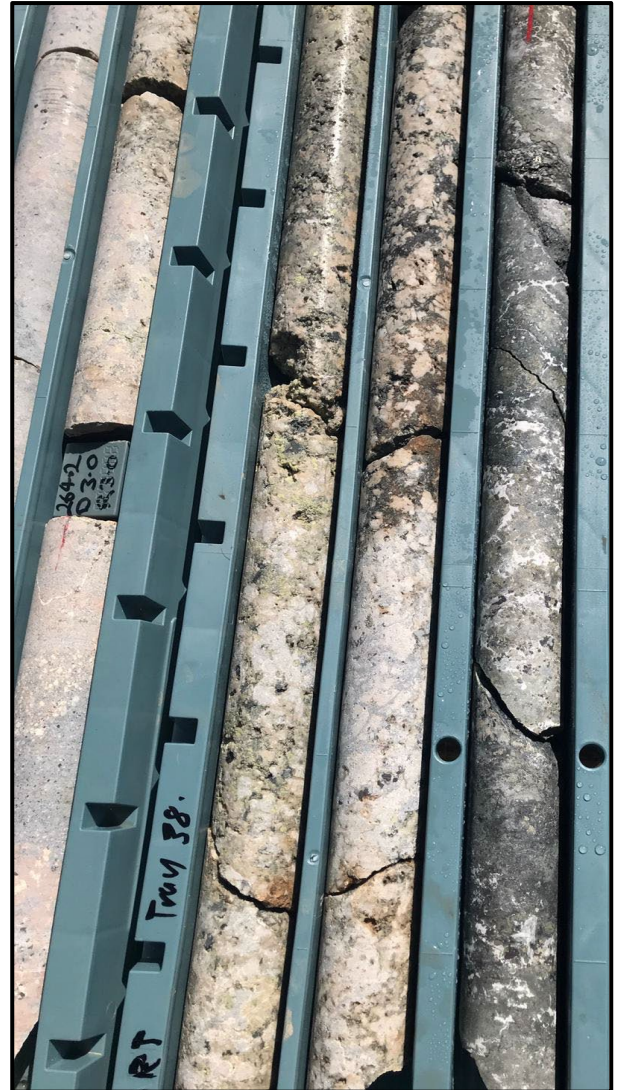
Figure 9. VK22DD01 264m to 267m: Brecciated dacite, strong epidote, chlorite, potassic alteration with visible sphalerite, galena, and pyrite.
