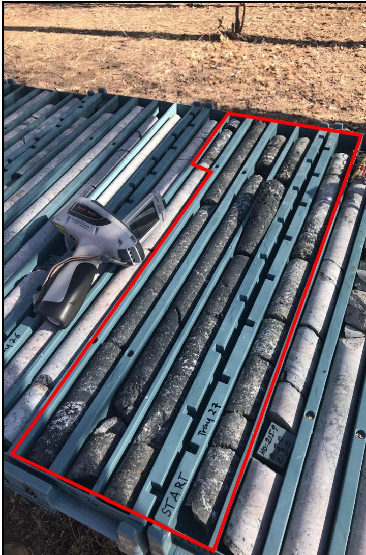
Figure 8. VK22DD01 211.95m to 215.96m: Dacitic unit with strong chlorite-carbonate alteration, visible sphalerite, galena, and chalcopyrite. To be sampled and submitted for assay.
