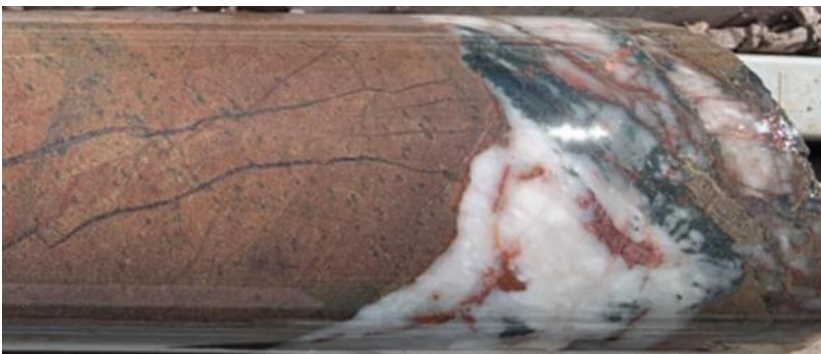
Figure 10: Quartz-chlorite hematite vein metamorphosed lithic sandstone. Hole depth: 338.4m.
