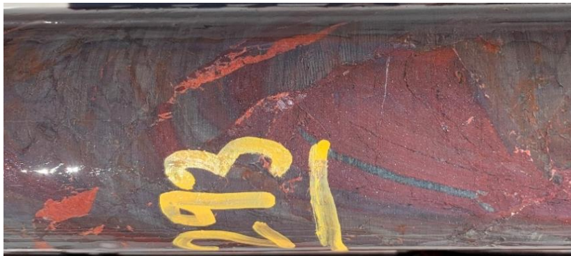
Figure 10: Faulted hematitic shale with later cross-cutting K-feldspar in-fill. Hole depth: 293m.
