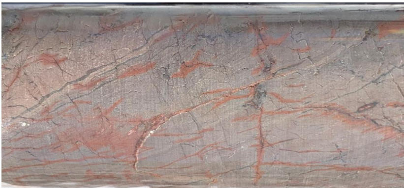
Figure 11: Hematite alteration 'bleeding' out from microfractures in metasediments. Hole Depth 298.7m.
