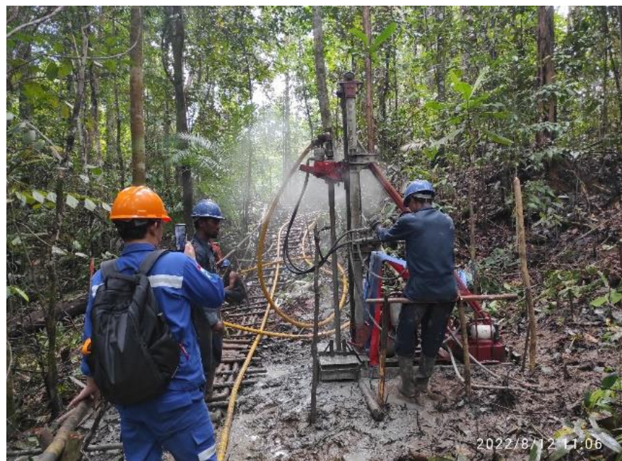
Photo 1: Compressor shot hole drilling operations
