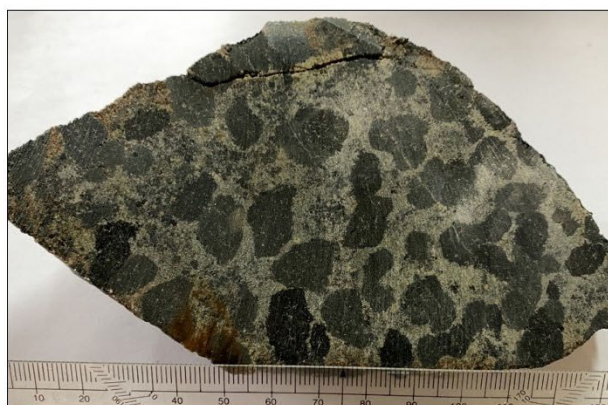
Photo 2: Ultramafic rock from outcrop with trace of chalcopyrite and pyrrhotite Sample G395828 (results pending). UTM 18 – NAD 83: 362,297 m E; 5,809,044 m N
