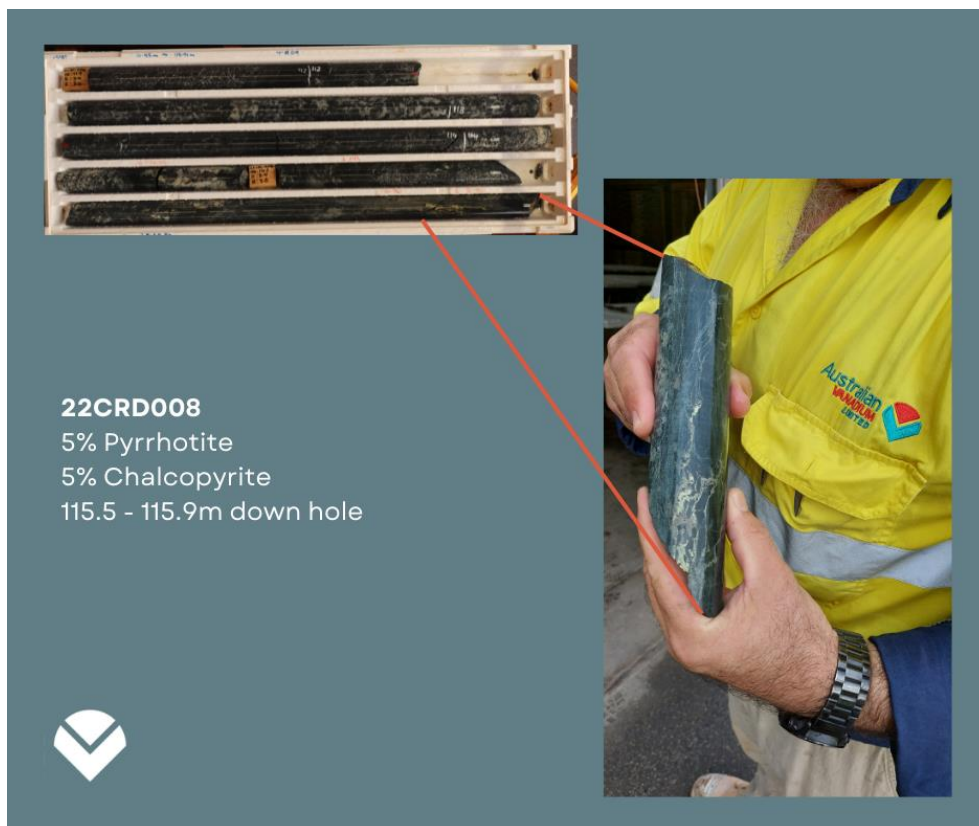
Figure 7 - Core photos of significant visual sulphide occurrences Top – 22CRD008 at 81.15m, Bottom 22CRD008 at 115.5m
